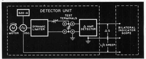
Figure 2. Block Diagram - Q Comparator.
