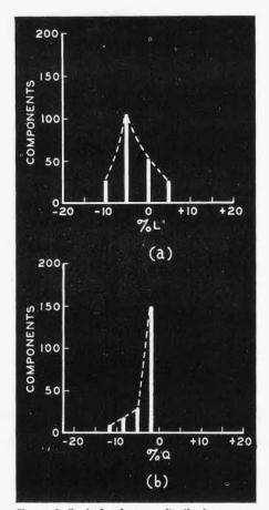
Figure 3. Typical tolerance distribution curves for analyzing pilot and production component runs.
